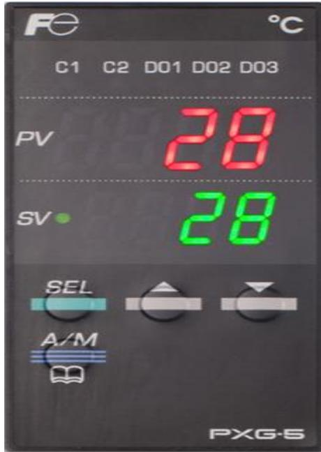
Embedded system with built-in PID algorithm, etc.
