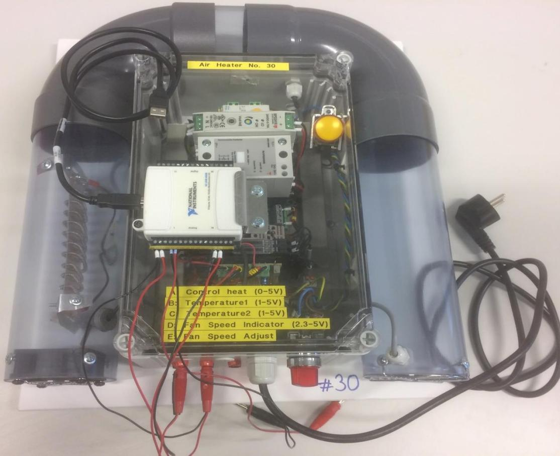
The Air Heater is a small-scale laboratory process suitable for learning about control systems
